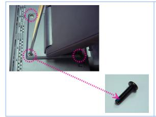
Remove 4 screws and then remove hinge.
